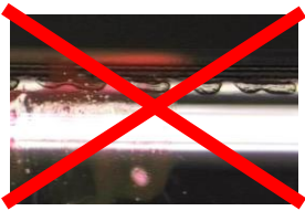
competitor = many bubbles size up to 400µm
